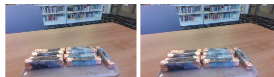
Figure 3. All samples with copper end caps, prepared for the C72 trial.
