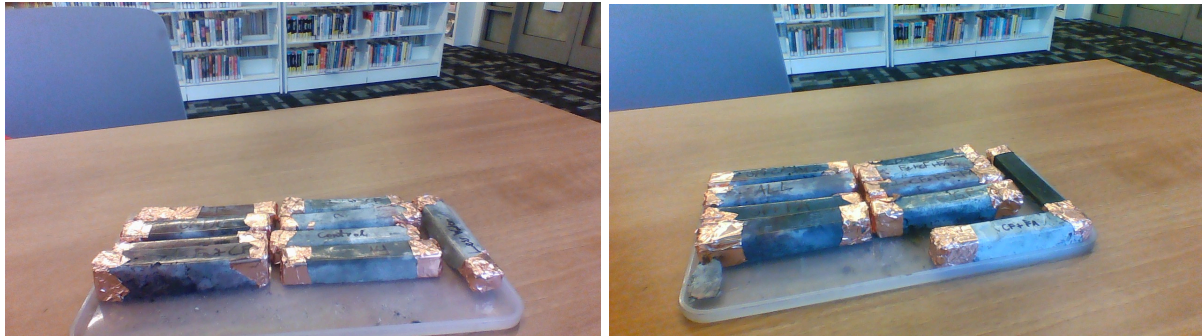
Figures 1 and 2 display our samples with copper foil end caps for the C72 and C32 trials. Photo taken by author on April 16th, 2026.
